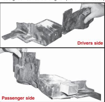
**13.** Notch plastic filler panel as shown in picture on each side and replace.
